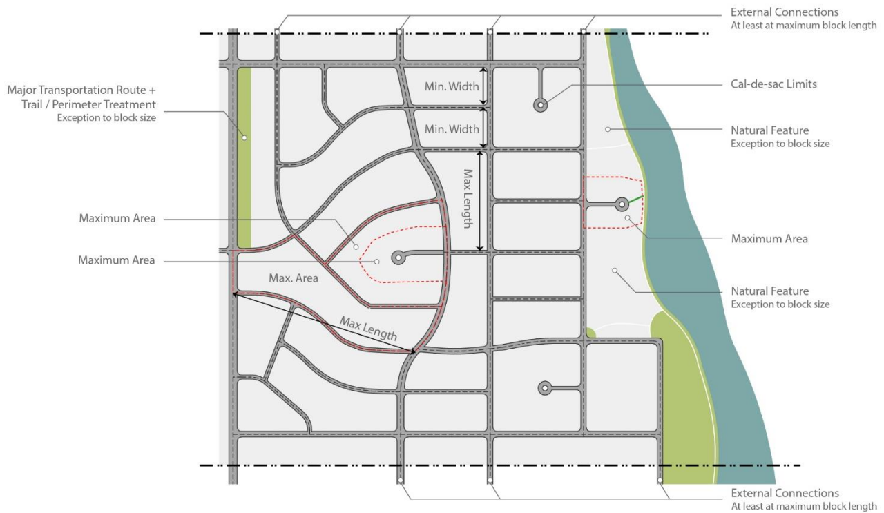
Figure 24-3-1 Connectivity & Block Sizes. Street networks shall be based on maximum block sizes (length between centerlines of perimeter streets and area) and stub to adjacent property at a frequency sufficient to create connected networks, unless exceptions justify not connecting.
