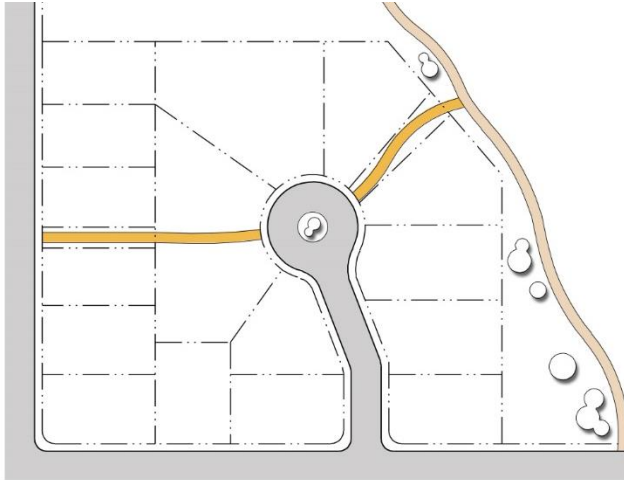
Figure 24-3-4 Walkways and Bicycle Routes. Where streets will not connect or where larger blocks are platted, connections for pedestrians or bikes may be required through blocks or at the ends of disconnected streets. (24-301.b.3).
